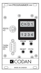
The CP-SC-3 synthesizer channel programmer is used to bench and field program the MT-3 family of synthesized radios. The CP-SC-3 synthesizer channel programmer is packaged in the same enclosure as the MT-3 receiver module, allowing it to be conveniently mounted in any receiver subrack slot position. An interconnect cable (Type F to DB-9) connects the front panel of the CP-SC-3 synthesizer channel programmer to any free standing synthesized receiver or transmitter, without disassembly.
